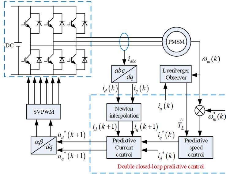
Fig. 1. Structural diagram of the double-closed-loop predictive control of PMSM
