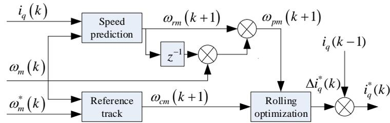
Fig. 2. Block diagram of PMSM speed ring prediction and control structure
